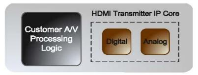
ASIC System-on-chip with Integrated HDMI Transmitter IP Core
